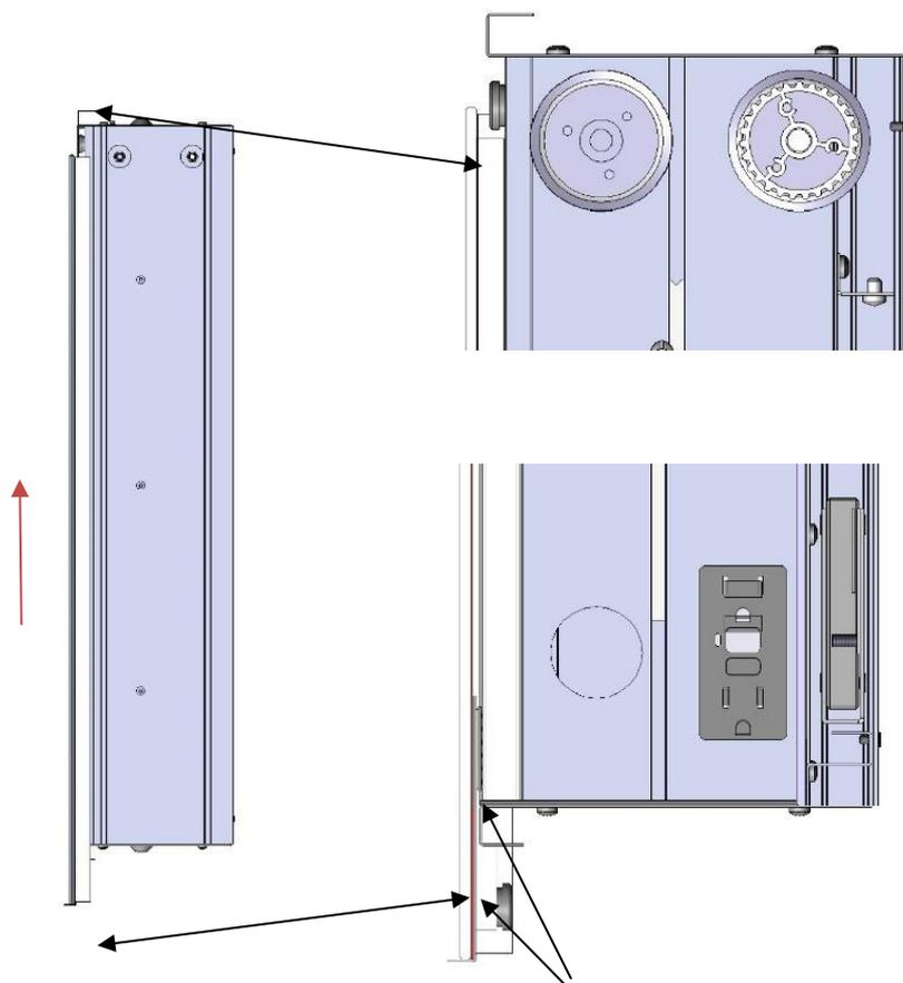
Watch out for the overhanging belt attachment on the mirror, not to damage the cabinet frame lip.
