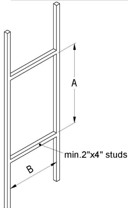
The framework should be prepared by a qualified tradesman. The cabinet can not be recessed into any insulated walls.
