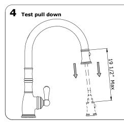
Ensure there is ample room in the space under the work surface for the hoses and weight to move freely. Test that the spray head extends far enough by pulling it out.
