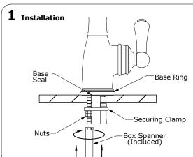
Before installing the product, leave a gap of 1 1/2" minimum from the center of the work surface hole to any walls or shelves (see image in section 5).
