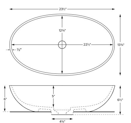
Base dimensions on counter top: 113/4" x 63/4" Always measure sink on-site to ensure cut-out accuracy.
