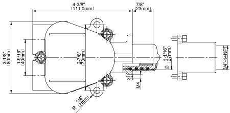
Three-Way Diverter Control Valve WITH Off Function (No Pass-Through) **G-8053**
