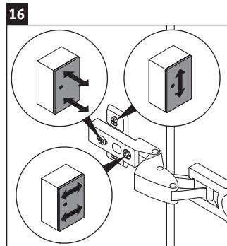
> The top screw will adjust up and down.
