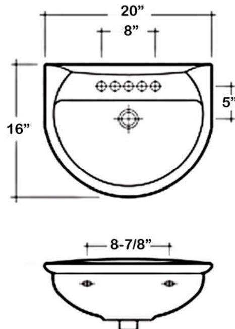
Dimensions of fixture are nominal and may vary within the range of tolerances established by ASME Standard A112.19.2.2018. Dimensions and specifications subject to change without notice.
