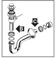
Secure lavatory on hanger as shown in 5. Insert and tighten anchor screws if applicable. Connect hot and cold supply lines to the shut-off valves. Tighten trap joints for watertight assembly. Apply a bead of caulk around the edge which contacts the wall as shown.
