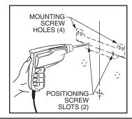
Affix hanger to wall (hand tighten only). Mount lavatory for positioning, level the deck, and mark bottom anchor screw holes (if applicable). Remove lavatory, tighten the hanger positioning screws and drill pilot holes for anchor screws and 4 mounting screws. Install and tighten the mounting screws.
